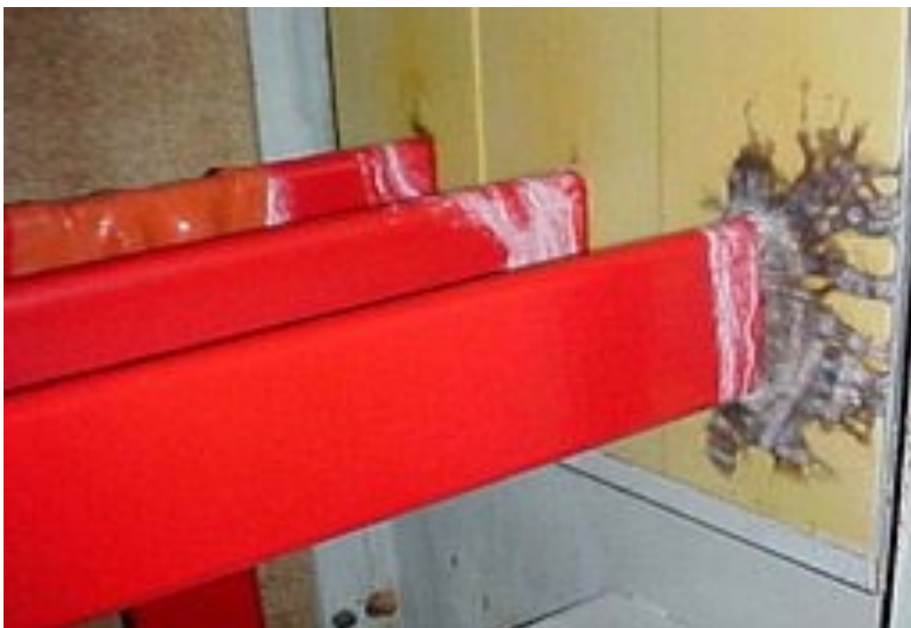
Partial discharge In Busbar Insulation
